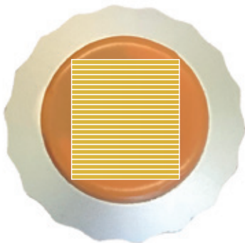
Illustration of the ceramic in a contact membrane linear array.
