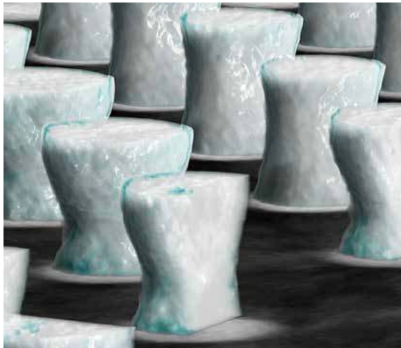
CL analysis of micro-bumps, defects on 60 µm bumps
