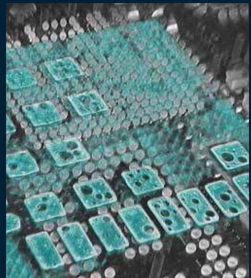
Computed Laminography of PCB, Clipping Plane
