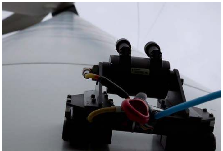
Remote Visual Inspection of a wind turbine
