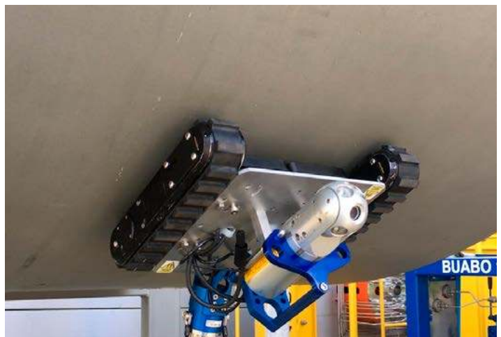
Curved steel wall inspection
